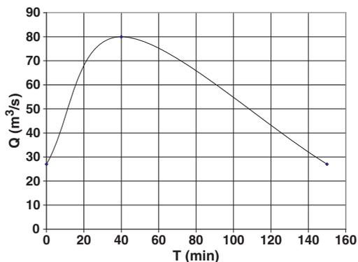
Figure 6 | Upstream inlet flow hydrograph in river.
