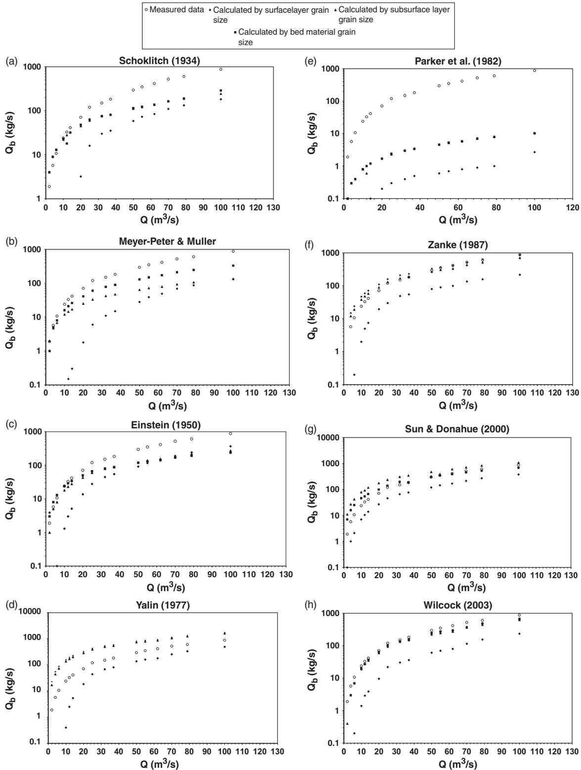
**Figure 15** | (a)–(h) Comparison of the results of bed load discharge formulas with measured data by using different grain size of bed layers.
